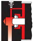
Sheffer's state-of-the-art cushion design features a unique, one-piece, nitrile compound seal that is captured within a precision machined groove. This allows both linear and radial "float" of the cushion seal which virtually eliminates problems associated with misalignment!
