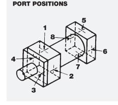
Ports are provided in positions 1 and 5. When a cylinder is cushioned, cushion adjusting screws will be located in positions 2 and 6. Cushion not available at head end of 1½" bore with 1" diameter rod.
